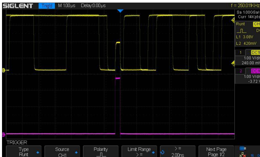
Figure 22 RUNT – Positive Polarity
