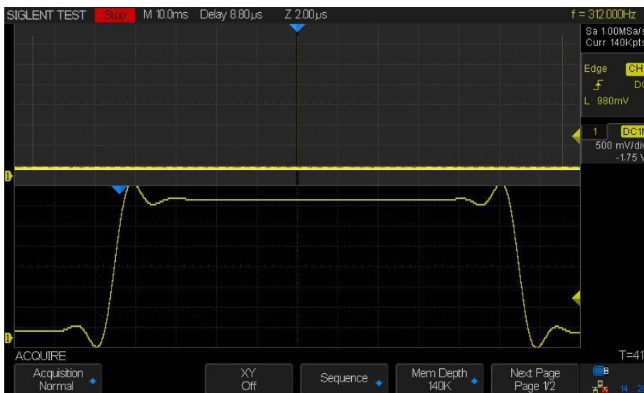
Figure 18 BURST - Short Recording Length, aliasing
