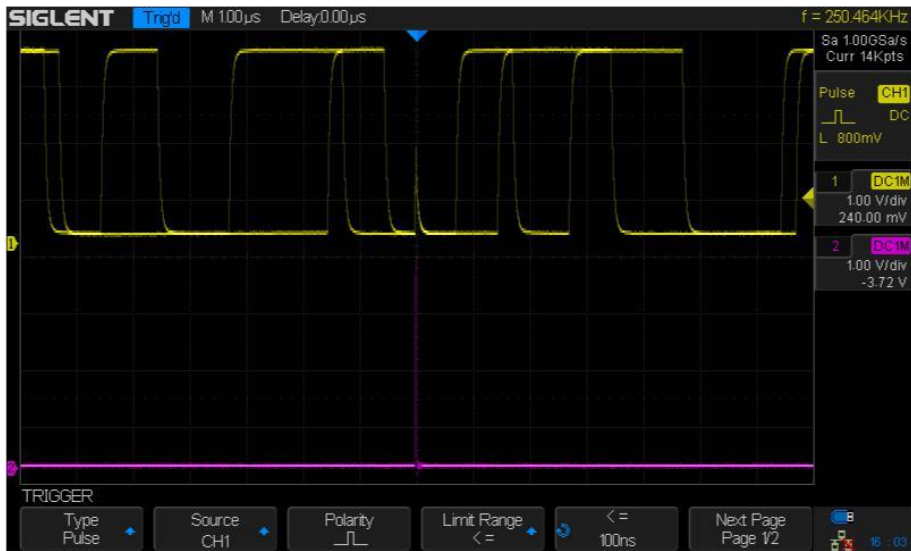
Figure 19 GLITCH – Positive Polarity
