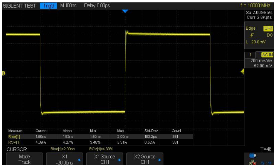
Figure 9 Fast Edge Square Wave – Using Ground Spring
