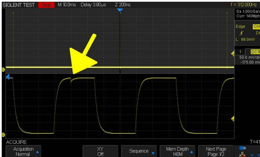
Figure 16 BURST – Long Recording Length, zoom in to see glitch detail
